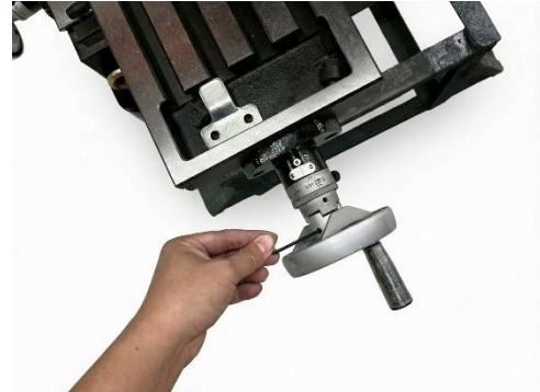
Figure 13: Installing the handwheels.
