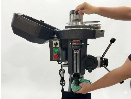
Figure 16: Tightening the draw bar.
