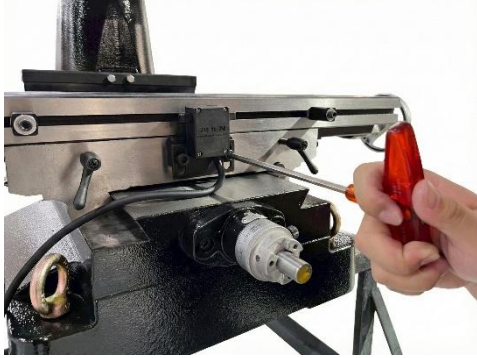
Figure 12: Installing the limit switch.
