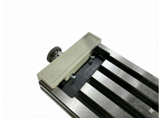
Figure 8: mounting the power feed bracket.
