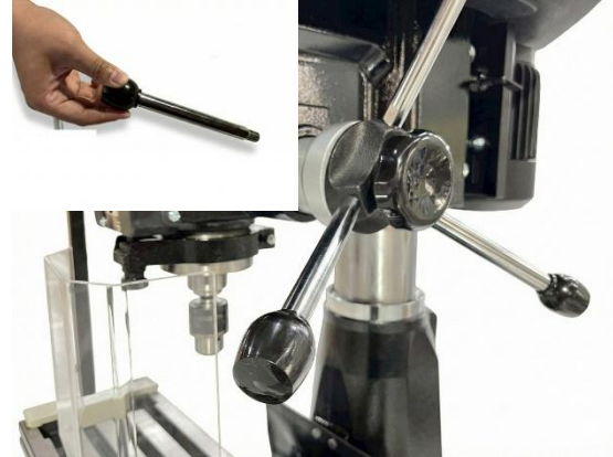
Figure 15: Installing the feed levers.
