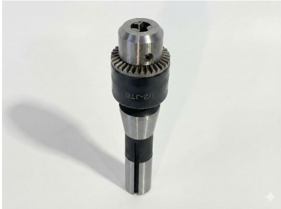
Figure 18: Joining The drill chuck and arbor.
