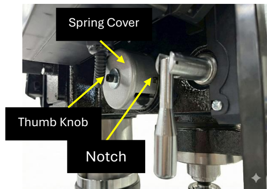
Figure 27: Return spring tensioning.
