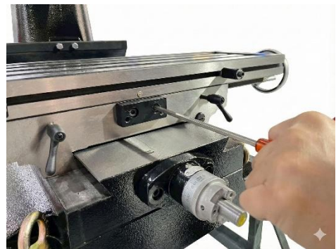
Figure 11: Installing the limit switch bracket.
