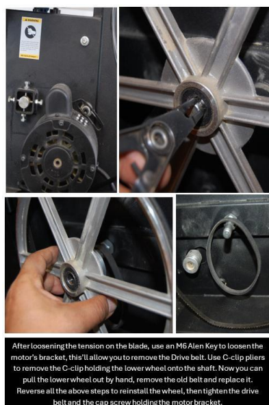
Figure 23: Replacing/ tensioning the drive belt.
