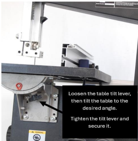
Figure 16: Table tilt mechanism.
