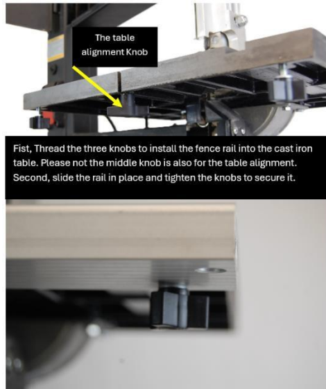
Figure 7: Installing the Rail and Fence.
