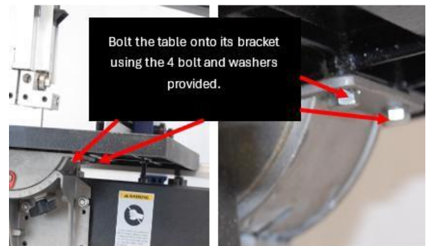
Figure 6: Assembling the Table.
