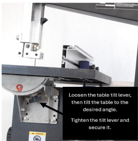
Figure 15: Table tilt mechanism.
