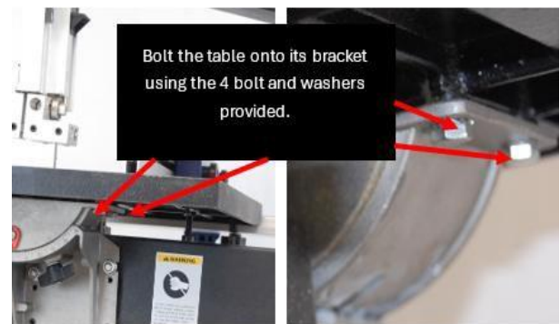
Figure 5: Assembling the Table.
