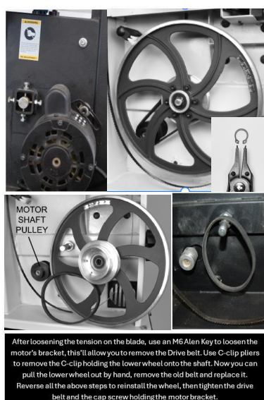
Figure 22: Replacing/ tensioning the drive belt.
