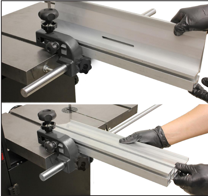
Figure 29: Changing the Fence to Horizontal
