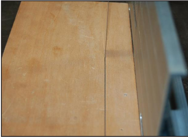
Figure 34: provides an example of a ripping operation, illustrating how the bandsaw is used for this task.
