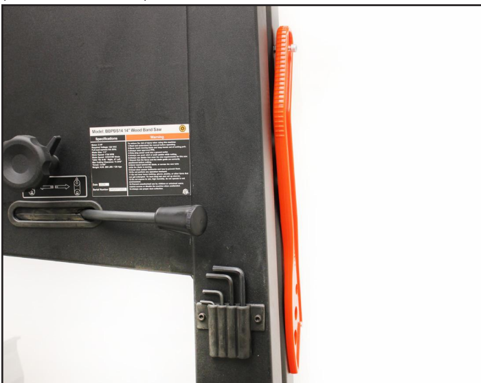
Figure 13: Installing the tool and Push Stick Holders.
