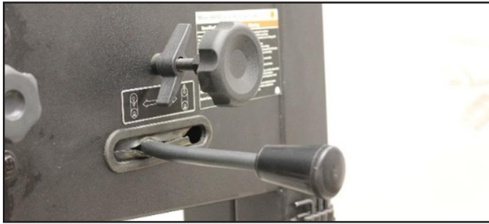
Figure 19: Blade Tracking mechanism.
