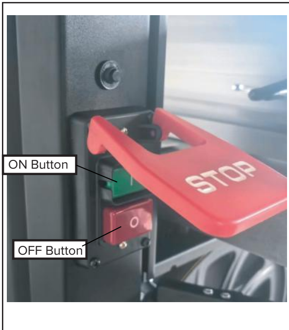
Figure 31: Main Switch Assembly.
