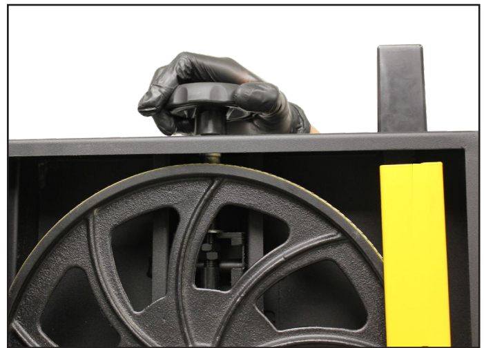
Figure 20: The Blade Tensioning Handwheel.
