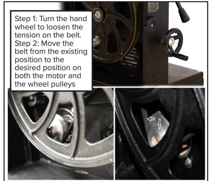
Figure 30: Changing the Band Saw Speed.
