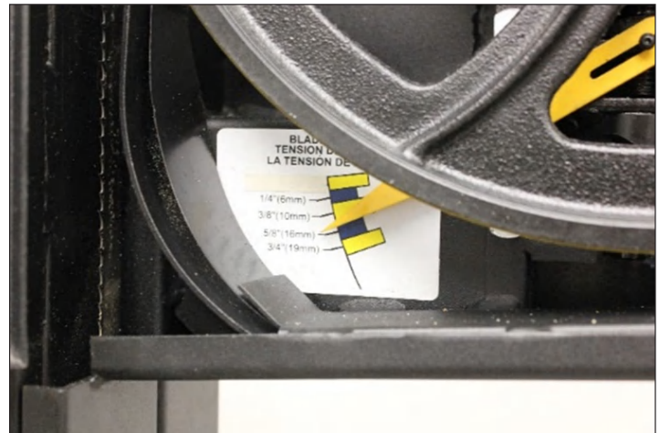
Figure 21: The Blade Tensioning Indicator.
