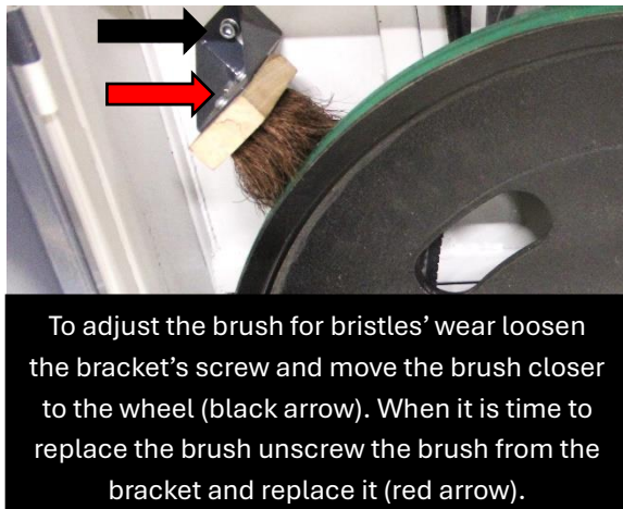
Figure 26: Wheel Brush Adjustment.
