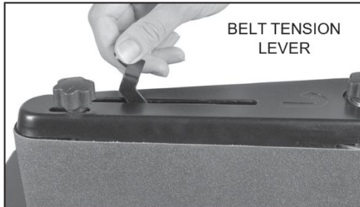
Figure 13: Tensioning Lever for the Belt.
