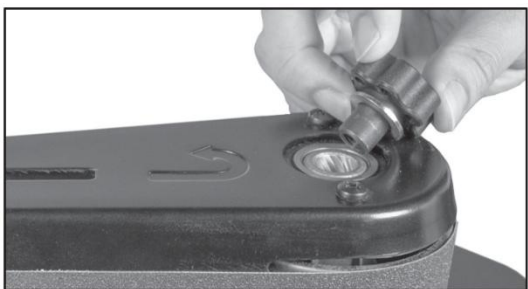
Figure 6: Tightening the Knob.
