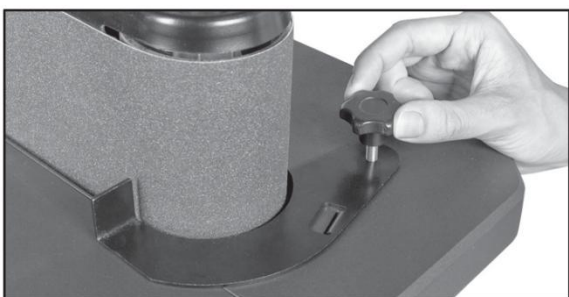
Figure 8: Installing the Limit Plate.
