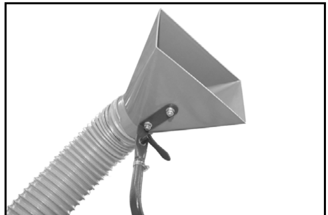
Figure-8 Securing dust hood to the bracket
