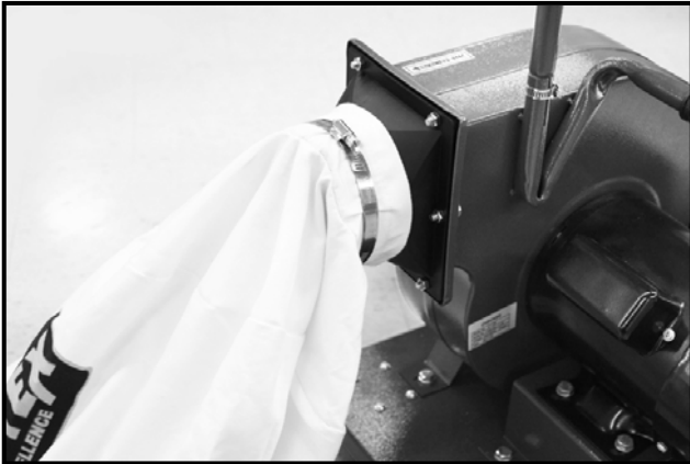
Figure-4 Installing the collection bag
