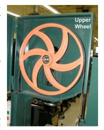
Center the blade on both the upper and lower wheels being sure that the blade runs through the upper and lower blade guides.
