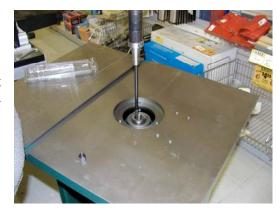
Install the spindle into the shaft as shown, being sure to engage the spindle locking detents. The spindle locking rod will protrude through the under part of the shaft. Use the locking rod nut to secure the assembly.
