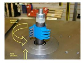
The B1363N includes both a 1/2" and 1/4" router bit adapter. Install the 1/2" adapter on the threaded spindle-locking rod and feed it through the shaft and lock it with the rod bolt.
