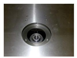
Remove the locking nuts (caution, the lowermost nut has conventional threads while the uppermost nut have reverse threads) from the top of the spindle and the required spacers to accommodate the shaper bit that you have selected. Re-install the locking nut. The installation should resemble the illustration.
