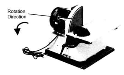
Before turning on the switch, please make sure to put on the flexible hose into the dust hood, 2-1/2"(63mm), and with hose clamp.
