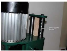
Square the hollow chisel with the fence by slightly loosening the chisel set-screw and using a tri-square, align the chisel.
