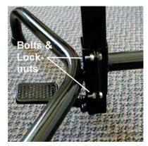
Remove the two bolts, flat washers and lock washers from the roller/ball assembly.
