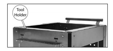
16.Fasten the table top into place using (4) M8-1.25 x 25 flat head screws and M8-1.25 hex nuts.
