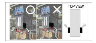
3. Turn on device to rotate and adjust the laser head until the red laser line is parallel with the drill bit.
