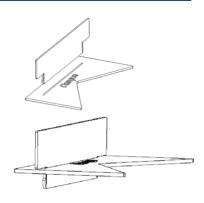
According to the direction and angle of I to be used, perpendicular to the scribinggauge, insert Auxiliary board into the rectangular hole of the scribing gauge, and makethe buckle lock Auxiliary board and the scribing gauge
