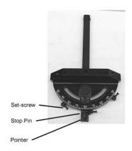
gauge from the slot and using an allen key, turn the stop set-screw to set the pointer to the 90 degree mark. The pointer is now accurate.
