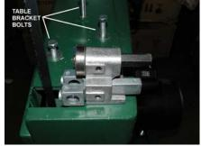
Fit the table trunions (already installed under the saw table) into the table bracket and tighten with the locking knobs.
