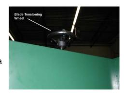
The blade tensioning control is found on the extreme top of the CT018. This is a wheel and turning it in a clockwise rotation will increase the tension on the blade. When the CT018 is not in use, the tension on the blade should be released to ease the pressure on the rubber tire and the bandsaw blade. By making this a habit you will extend the life of the rubber tires and the wheel bearings.
