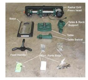
Some of your Craftex drill press components have been coated with a protective lubricant to prevent rust. Prior to assembly, these parts should be cleaned with a soft cloth dampened with mineral spirits. When cleaned, the components should be coated with paste wax and then buffed dry.
