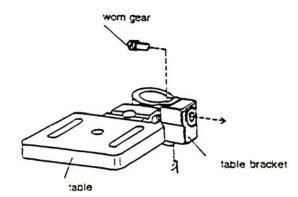
Place the rack into the table bracket and link it with the gear, the bottom end of the rack should be inserted into the groove on the column base and tightened.
