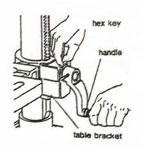
Mount the clamping lock on the rear of the table bracket.
