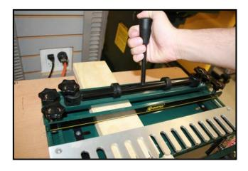
Figure 5 shows clamping down the work-piece
