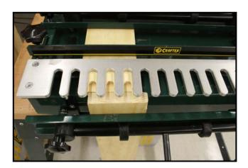
Figure 11 shows dovetails after cutting
