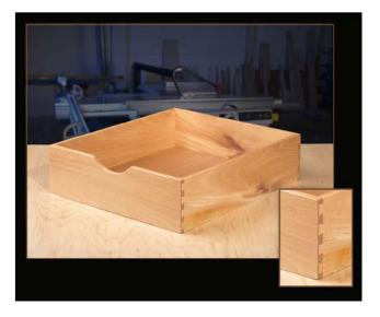
Figure 12 shows a finished drawer and 2 sides ready to be joined
