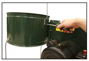
Attaching Top Bag Support Bar to the Collector
