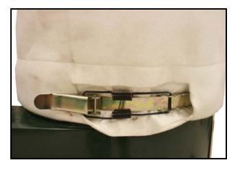
Top Filter Bag Attached to the Collector
