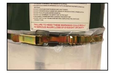
Bottom Bag Attached to the Collector
