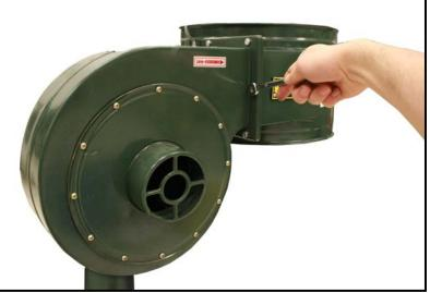
Attaching Collector to the Motor/Impeller
