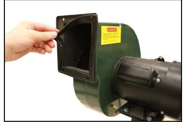
Attaching the Gasket to the Impeller Opening
