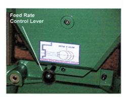
If a board jams, immediately set the gearbox to 'neutral', turn off the power and release the
