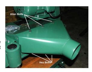
Three additional hex bolts are provided to secure the bottom flange of the Dust Hood in the threaded holes provided.
