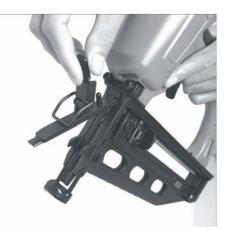
The exhaust deflector can be positioned to point in any direction (Full 360° movement) Reposition deflector by grasping firmly and rotating the desired position.
