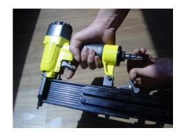
2. Insert fasteners into magazine. See over leaf for details. Then shut magazine by pushing fully upwards.
