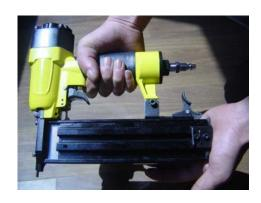
3. Check air supply is at least 60 PSI. The gun is now ready to use. Press the head of the gun onto the work piece to be fastened and squeeze the trigger to fire nail.
