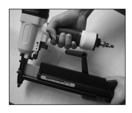
3. Check air supply is at least 60 PSI. The gun is now ready to use. Press the head of the gun onto the work piece to be fastened and squeeze the trigger to fire nail or staple.
