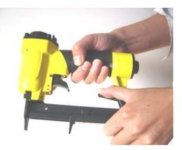
2. Insert fasteners into magazine. See over leaf for details.Then shut magazine by pushing fully upwards.
