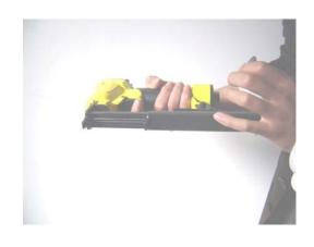
3. Check air supply is at least 60 PSI. The gun is now ready to use. Press the head of the gun onto the work piece to be fastened and squeeze the trigger to fire staples.
