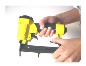
2. Insert fasteners into magazine. See over leaf for details. Then shut magazine by pushing fully upwards.
