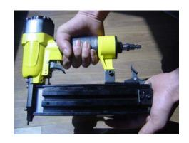
3. Check air supply is at least 60 PSI. The gun is now ready to use. Press the head of the gun onto the work piece to be fastened and squeeze the trigger to fire nail.
