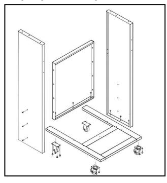
Figure-5 Installing the stand supports
