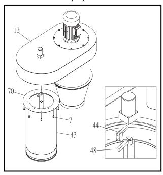
Figure-6 Installing the canister filter
