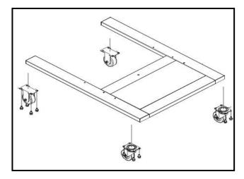
Figure-4 Attaching wheels to the base
