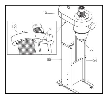
Figure-7 Installing the main housing
