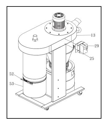
Figure-9 Installing the magnetic switch
