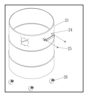
Figure-8 Installing the collection drum wheels
