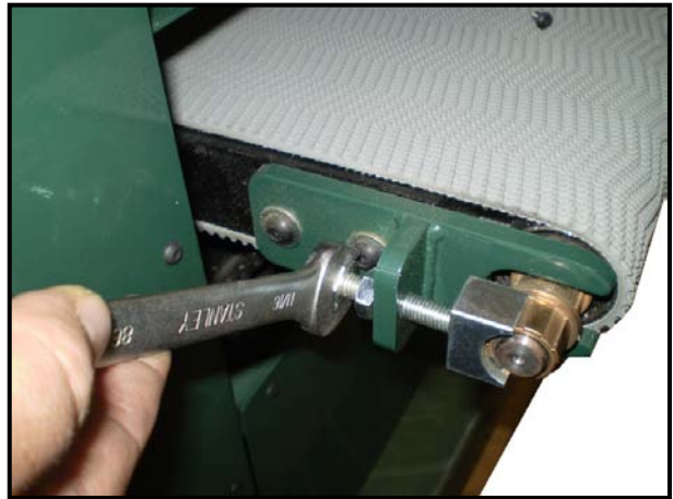
Figure-11 Tracking Conveyor Belt
