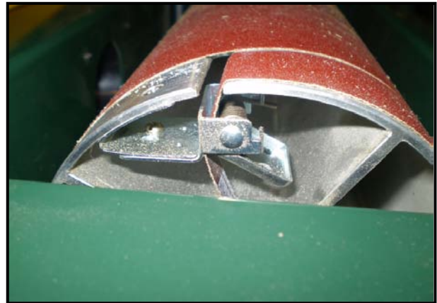
Figure-9 Spring Loaded Quick Release Mechanism
