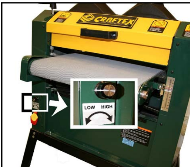
Figure-9 Speed Knob Control
