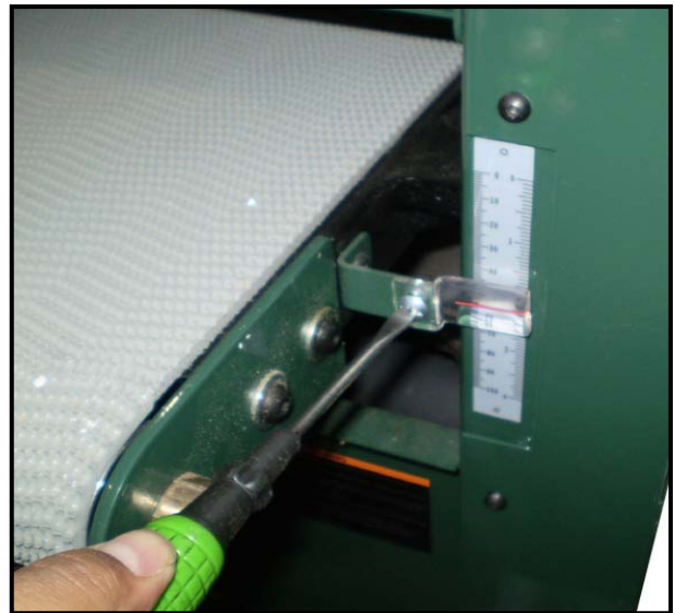
Figure-11 Calibrating the Thickness Scale
