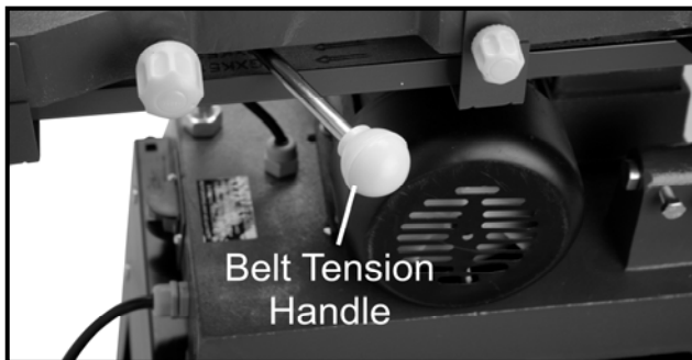
Figure-23 Loosening the tension on the belt
