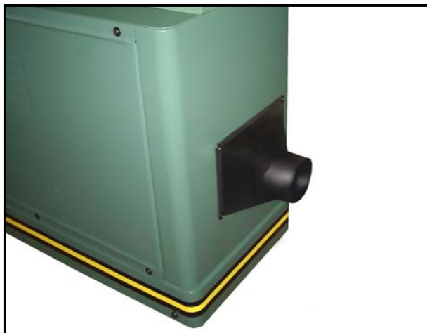
Figure 9: Installing dust hood
