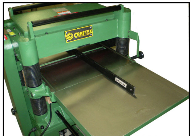
Figure-7 Leveling the wings using straight edge
