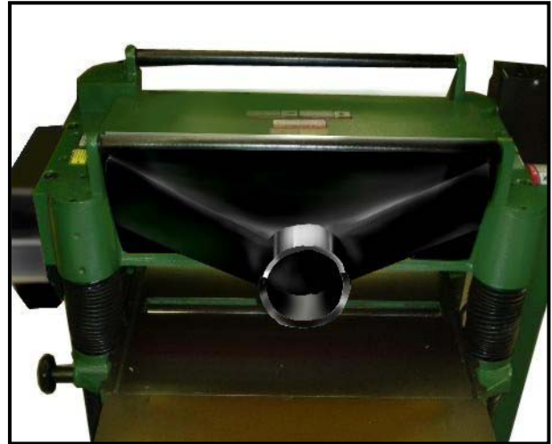
Figure-9 Attaching the dust hood
