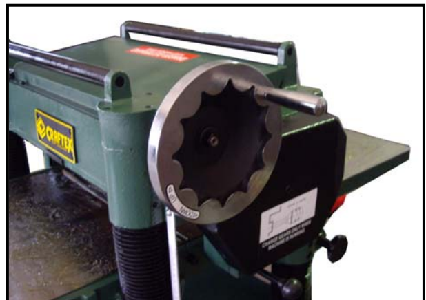
Figure-10 Installing the hand-wheel
