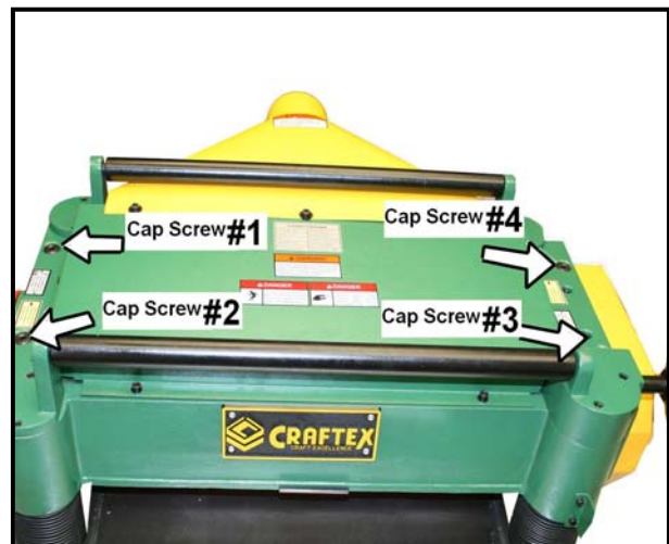
Figure-23 Set screws for the roller spring tension adjustment
