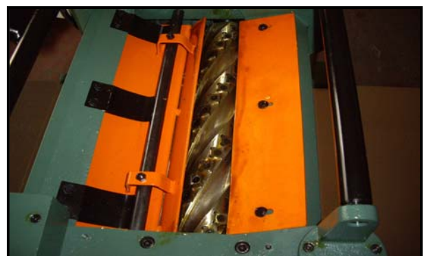
Figure-21 Cutter-head exposed
