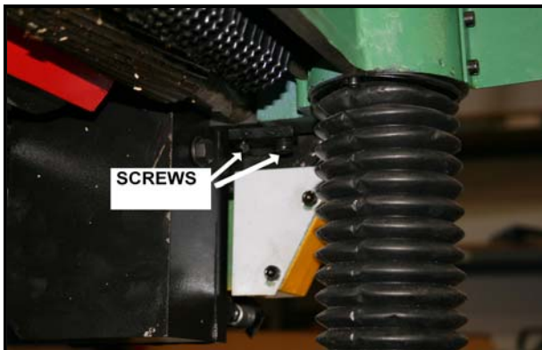
Figure-16 Setting the rollers spring tension
