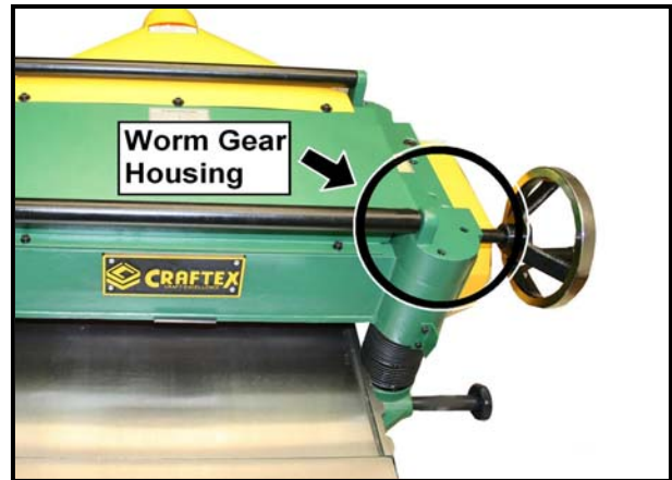
Figure-25 Worm gear lubrication location
