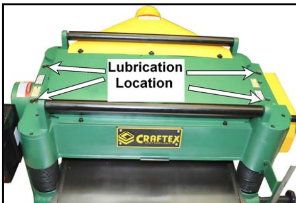
Figure-24 Lubrication holes for the feed rollers
