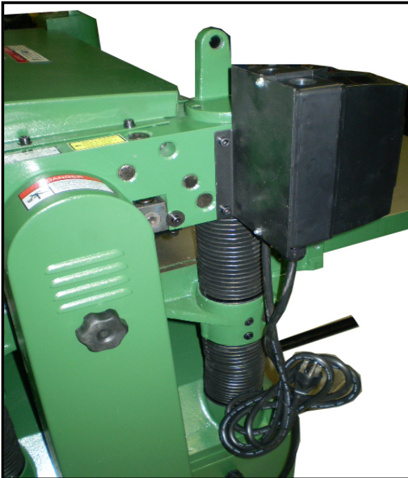
Figure-8 Installing the magnetic switch
