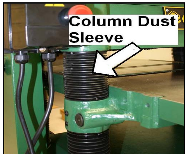
Figure-26 Column dust sleeve
