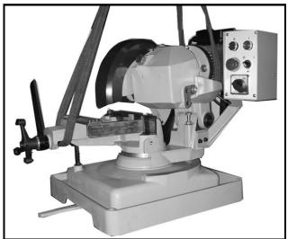
Figure-2 Lifting straps around the motor and the jaw of the CX110
