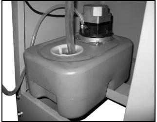
Figure-12 Coolant tank inside the stand
