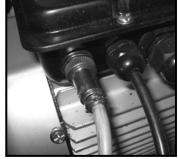
Figure-7 Connecting the cable to the socket
