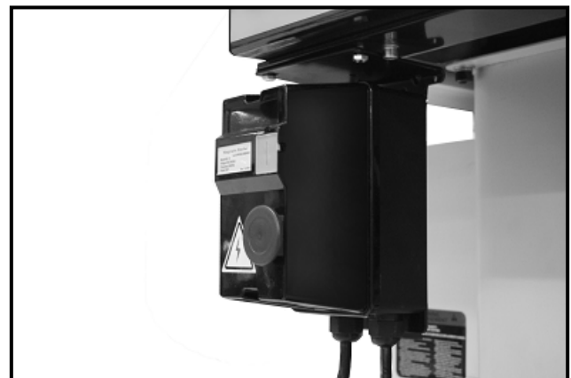
Figure-21 Installing the magnetic switch
