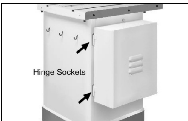
Figure-7 Installing the cabinet door
