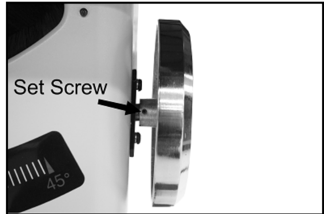
Figure-8 Securing the blade tilt hand wheel
