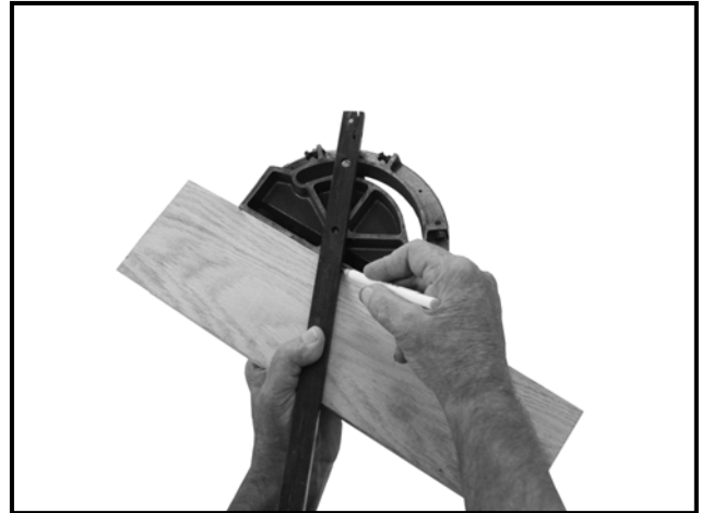
Figure-34 Marking the angle of cut
