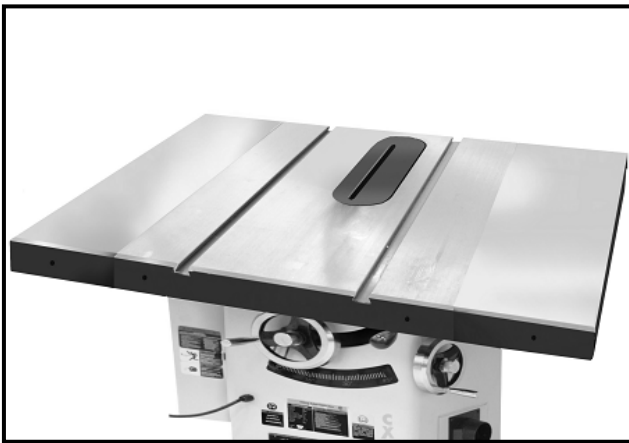
Figure-11 Installing the extension wings
