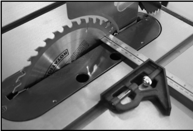
Figure-35 Measuring the distance using an adjustable square
