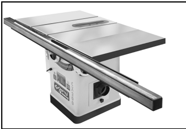
Figure-15 Installing the fence rail tube
