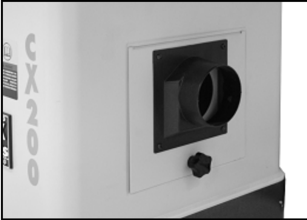
Figure-10 Installing the dust port
