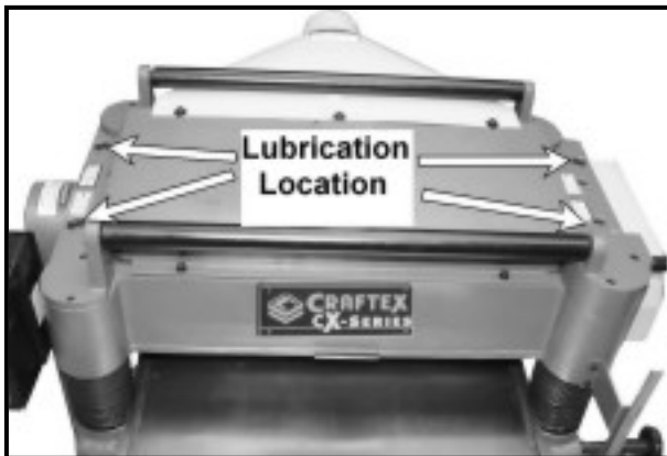
Figure-24 Lubrication holes for the feed rollers
