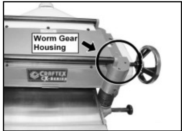
Figure-25 Worm gear lubrication location
