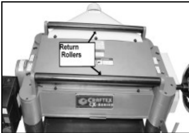
Figure-19 Top return rollers
