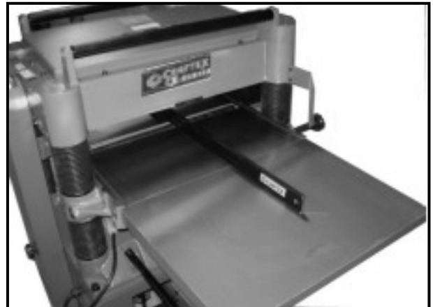
Figure-7 Leveling the wings using straight edge
