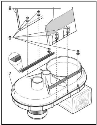
Figure-2 Fan housing
