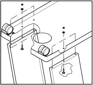
Figure-6 Attaching the bottom panel to the side panels
