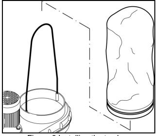
Figure-8 Installing the top bag
