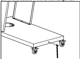
Figure-5 Threading the earth-chain
