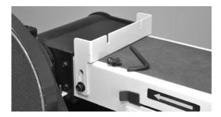
Figure 2 – Install the small fence.
