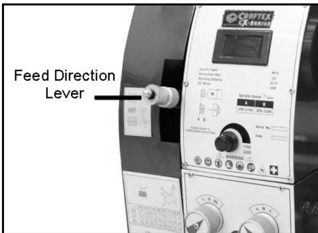
Figure-20 Feed direction selector knob
