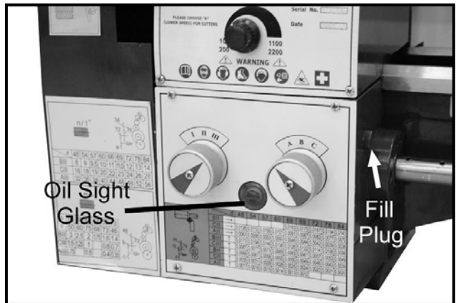
Figure-40 Fill plug location
