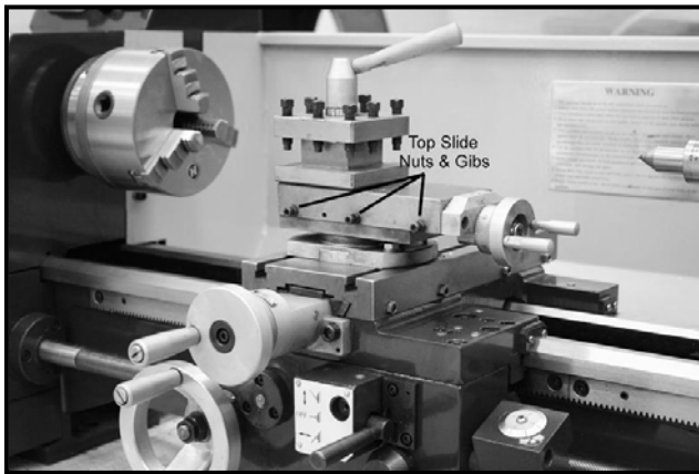
Figure-32 Top slide adjustment gibs screws
