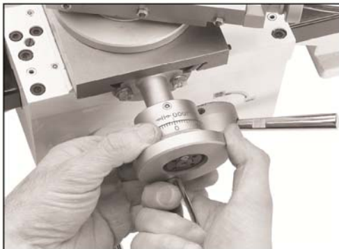
Adjusting handwheel scale.
