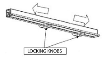
2. Position the guide fence firmly on to the guide fence rail and press the handle down to lock it in place.
