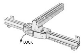
3. Place the fence on the table and hold in place using a clamp preferably. Space the mounting brackets as far apart as possible then tighten the locking knobs. Press the assembly to the front edge of the table top and using a marking tool or centre punch mark the holes from the moutning brackets.
